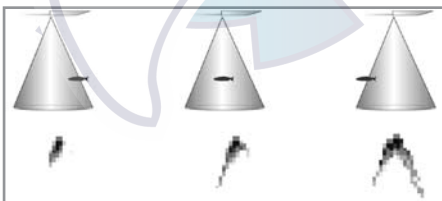
Transducer Cone and Fish Arches
